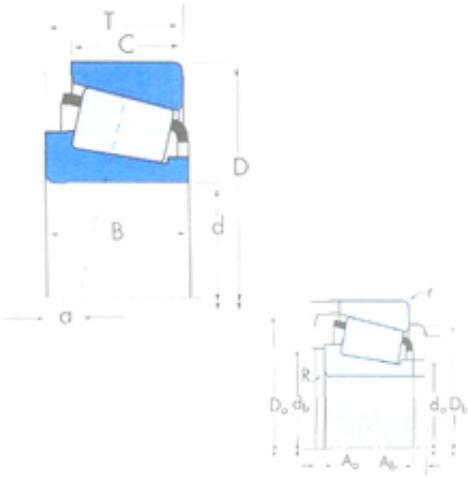
M88048/M88010 Bearing 2D drawings and 3D CAD models
